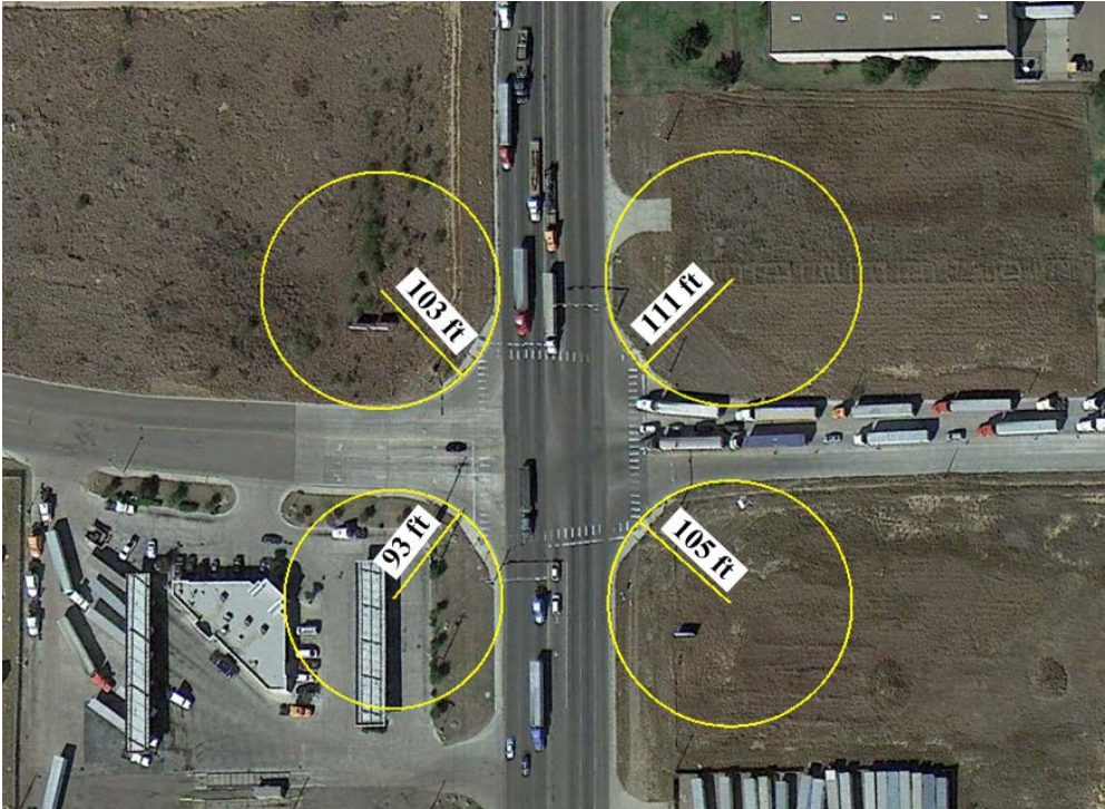
Figure 12. Approximate Radius of Each Right-Turn Approach at the Intersection of Mines Road and Killam Industrial Boulevard (Source: Google Earth.)
