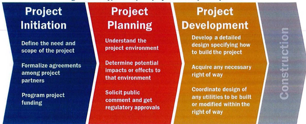
Figure 18 – Typical capital project development process
