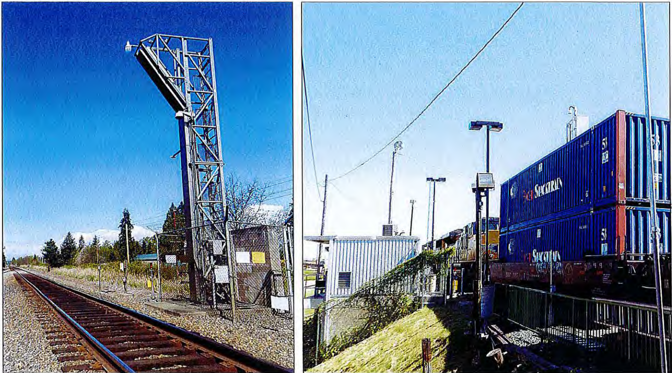
Figure 3: R-VACIS in Blaine, Washington, (left) and a train proceeding through R-VACIS in Laredo, Texas (right)
