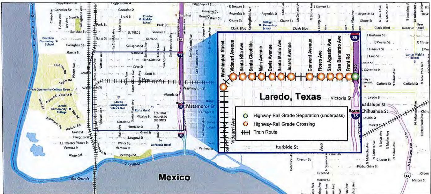
Figure 8: Selected Highway-Rail Grade Crossings in Laredo, Texas
